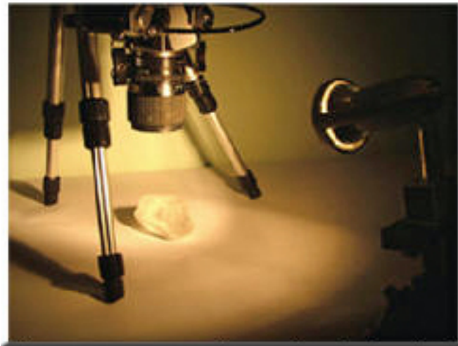
A film camera mounted on a tripod and pointing down at an illuminated crystal.
