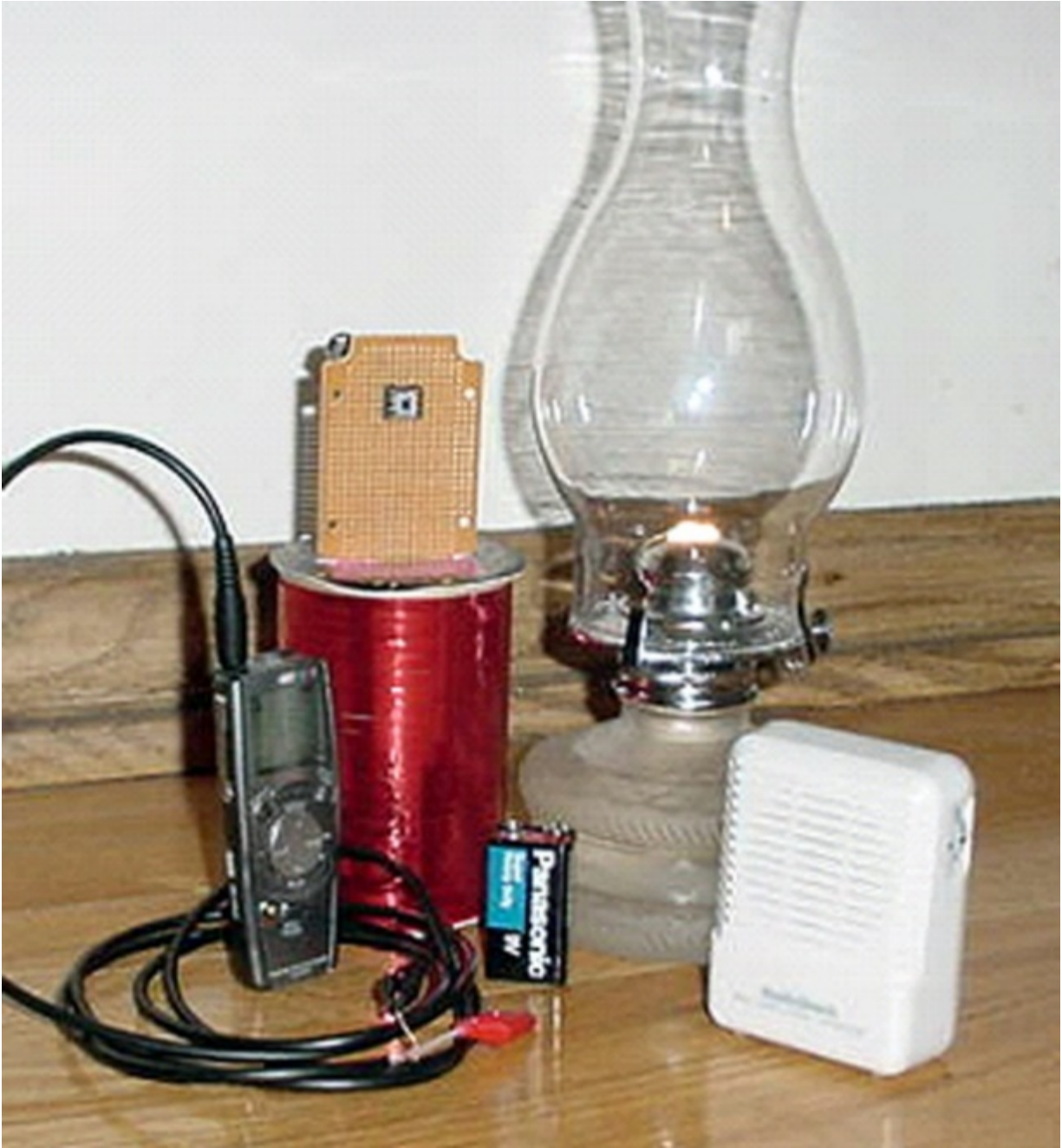
Oil lamp light source, optical detector/amp mounted on “breadboard” material. Audio recorder connected at “microphone in” with cable equipped with two “alligator clips.” The small white box is the Radio Shack mini amp.
