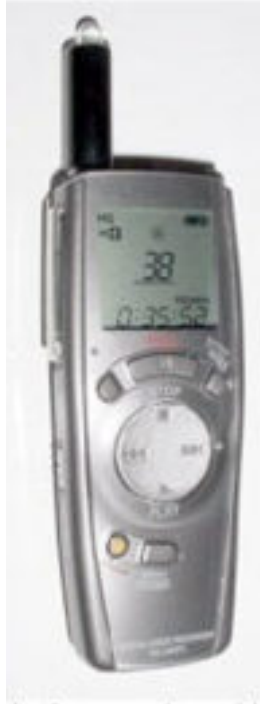
Audio recorder with detector mounted in microphone jack
